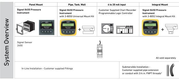
\*Refer to the Signet Submersion Kit brochure (3-0000.707) located on our website for installation suggestions and options. 8058 signal converter and 8059 external relay module also compatible
